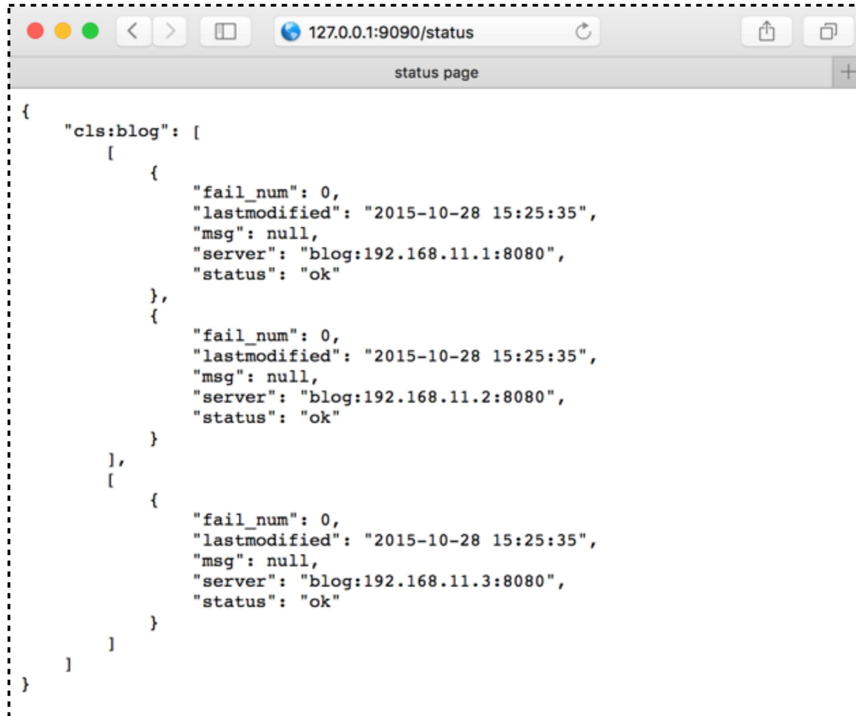
The image shows a browser window with the address bar containing "127.0.0.1:9090/status". The page title is "status page". The content of the page is a JSON object representing the status of three upstream servers. Each server entry includes a failure count, a last modified timestamp, a message, the server address, and a status.
